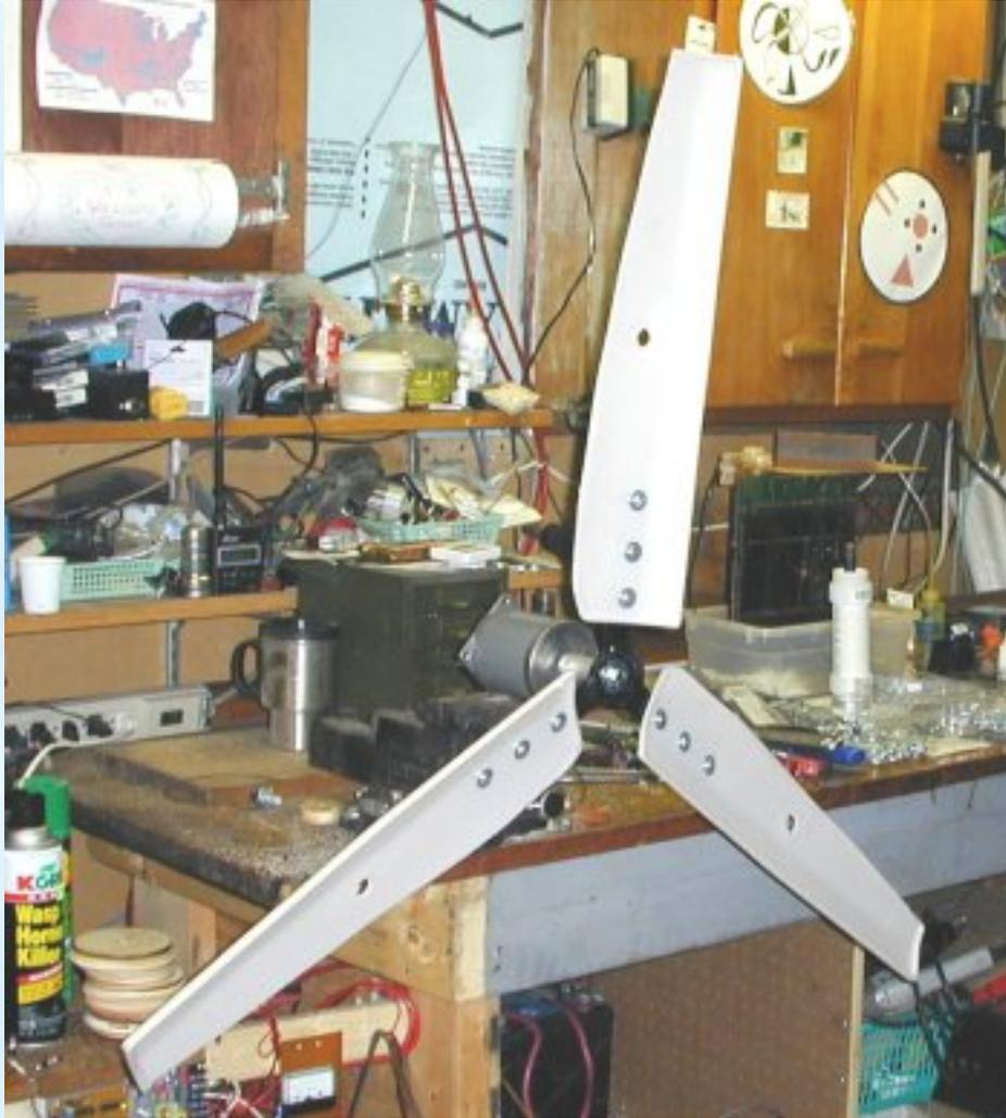
The three steel strips were marked and drilled, then tapped for three 1/4"-20 screws in each one to mount the blades. At this time I also scribed a line an inch out from the washer across each one. Each strip was then clamped in the vice at this line, and using a large crescent wrench I twisted each one to the proper blade angle, sighting it with another line drawn across the top of the vice with magic marker.
