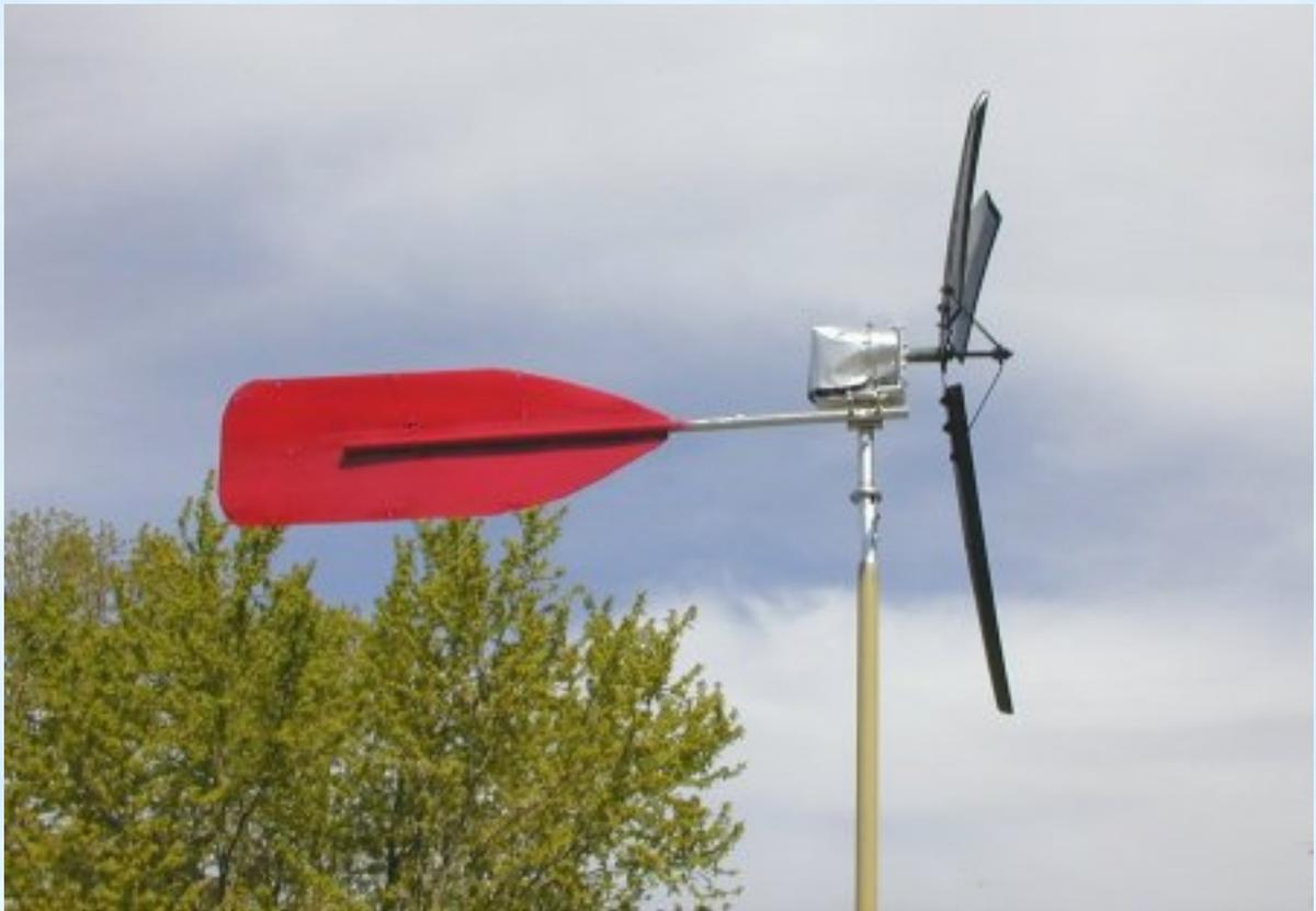
This side view shows the forward rake of the blades. This should allow plenty of room for flexing in extreme weather.
