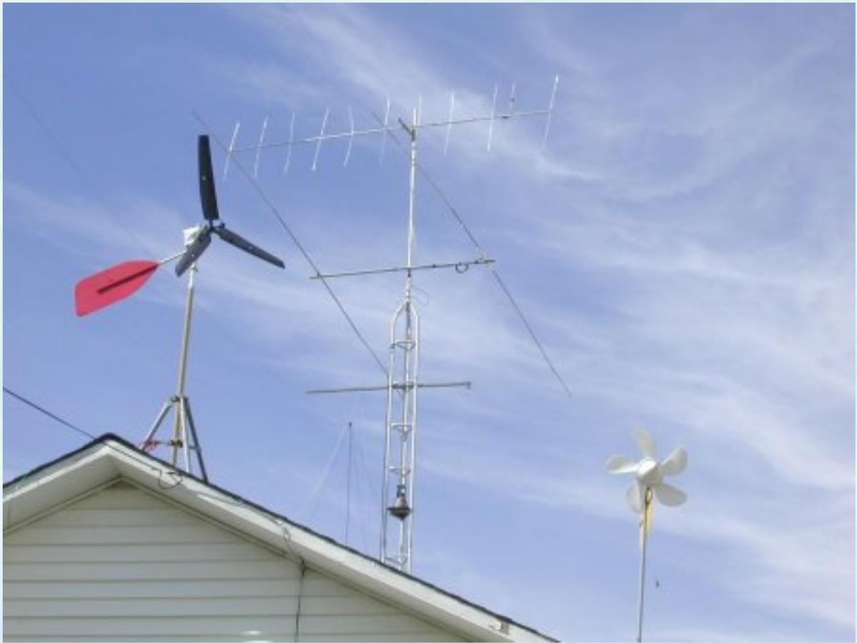
Here it is, up on the shop roof. To the right is the original Microwind prototype, fastened to the vent pipe where it's been adding it's share to the station batteries for over a year now. I've seen an amp out of the little guy, and I hope the bigger version will do much better.
