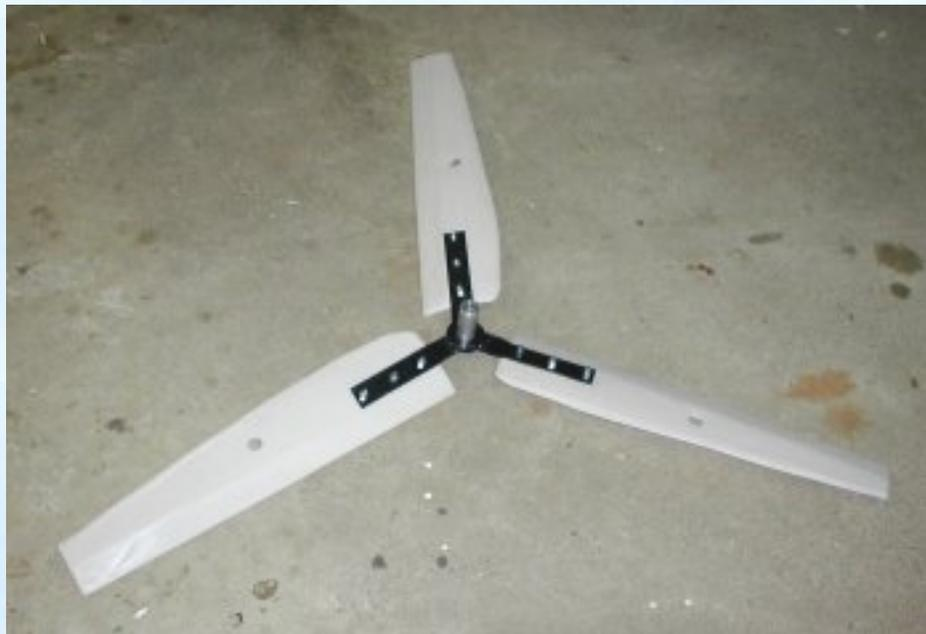
I found a scrap of heavy gauge steel about 1 1/2" wide, and cut it into three equal strips about 7 inches long. These I sandwiched between two very large washers. A bolt and nut squished the washers together, capturing the steel strips. Once they were perfectly aligned, I welded them all together, forming a solid three-blade hub.
