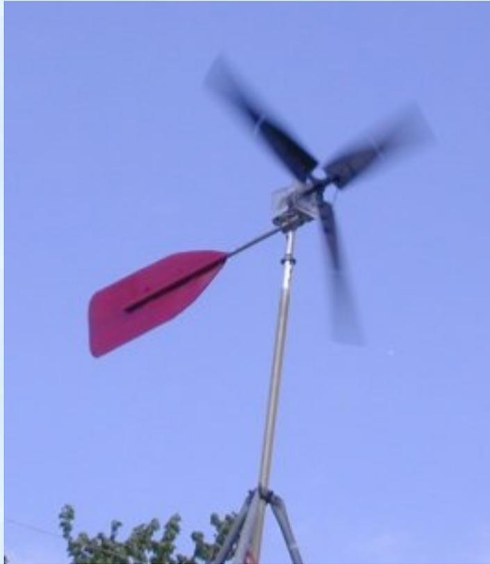
The result is a bit more speed in the gusts. As I write this we're having winds with gusts up over 20 mph, and I'm seeing an easy 1 to 1 1/2 amps going into the batteries on the average, more in the strongest peaks. This is certainly not bad for a little NEMA 34 stepper motor. I have a feeling that it will do better in some real wind, at least as long as it holds together.
